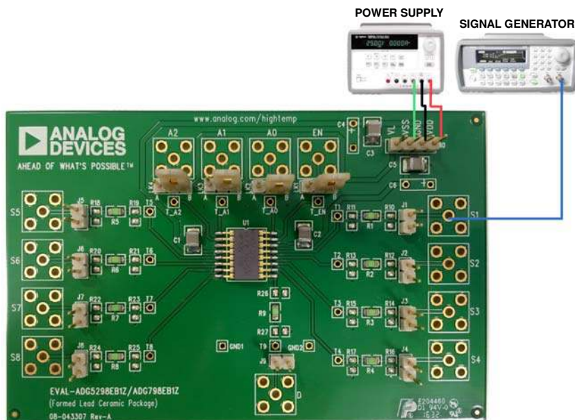
Figure 1. EVAL-ADG5298EB1Z , Power Supply, and Signal Generator
