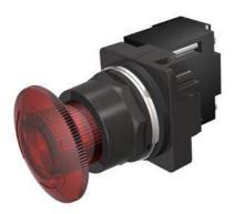
30mm BlackMax, Epoxy Coated Corrosion Resistant Metal Operator, Round Illuminated Twist-to-Release Transformer type, 600V AC LED Lamp Mushroom Head Cap Small 1.79" (45 mm) Plastic Cap, Red 2 Position Maintained, Twist-to-Release UL Listed, CSA Certified NEMA 1,3,3R,4,4X,12,13 & Automotive Standards
