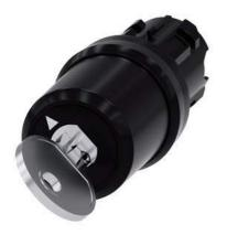
key-operated switch Siemens, 22 mm, round, plastic, lock number SSG10, with 2 keys, 2 switch positions O-I, latching, actuating angle 90°, 10:30h/13:30h, key removal I, with laser labeling, inscription or symbol customer-specific selection with SIRIUS ACT configurator (CIN)
