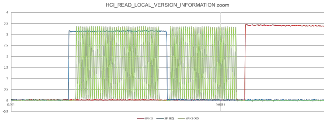
Figure 21. HCI_READ_LOCAL_VERSION_INFORMATION SPI waveform zoom
