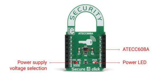
The device is consuming very low current, especially while it is in the sleep mode. The chip itself uses less than 150nA, in that case. The voltage range which can be used to power up the Security 4 click, allows for it to work with both 3.3V and 5V capable MCUs.
