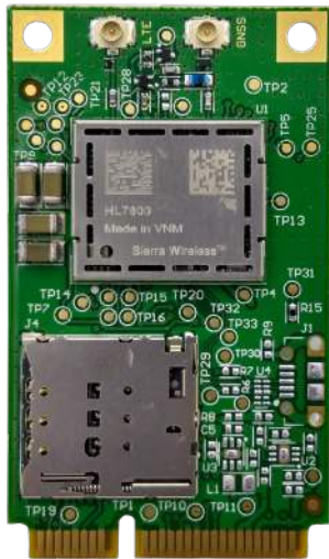
CellCracker mPCIe card LTE modem
