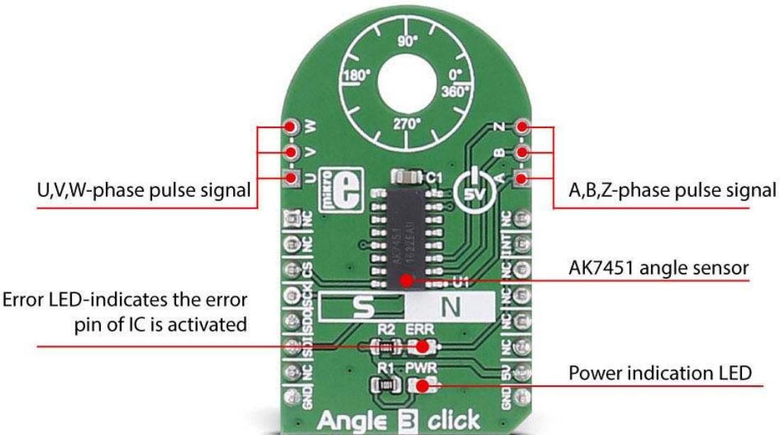
There are 3 output pins on board (A, B, Z) where the IC outputs pulses for the encoder feature and the 3 output pins (U, V, W) where the IC outputs pulses for the BLDC motor drive.
