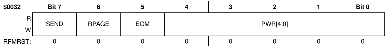
Figure 100. RFM Control Register 2 (RFCR2)
