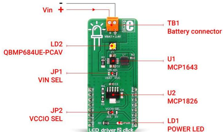
The LED brightness can be regulated by applying a variable duty cycle PWM signal to the EN pin of the MCP1643 regulator (routed to PWM pin on the mikroBUSTM). This results in changing the current running through the LED in a linear fashion, from 0 to the value set by the resistor, depending on the PWM cycle.
