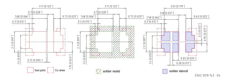
For superior solder joint connectivity results we recommend soldering under standard nitrogen atmosphere. Package not suitable for ultra sonic cleaning.
