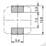
no sensitive traces underneath the component
