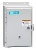
Non-reversing motor starter, Size 0, Three phase full voltage, Solid-state overload relay, OLRelay amp range 3-12a, 240V 50HZ / 277V 60HZ coil, Non-combination type, Enclosure type 12, Dust/drip proof for indoors, Extra-wide enclosure
