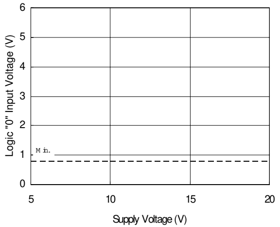
Figure 9B. Logic "0" Input Voltage vs. Supply Voltage
