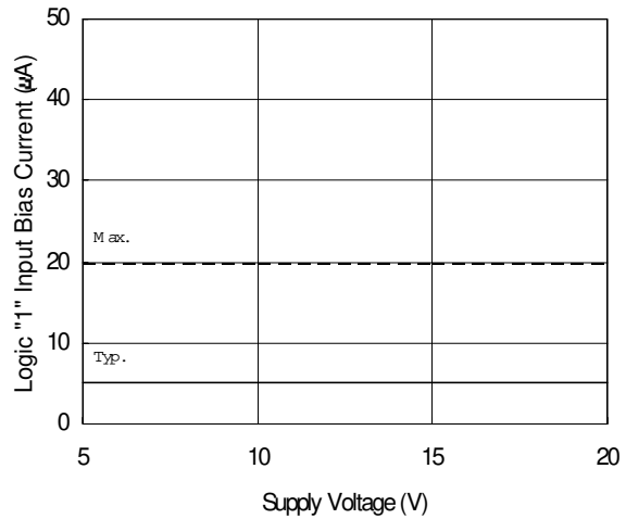
Figure 15B. Logic "1" Input Bias Current vs. Supply Voltage
