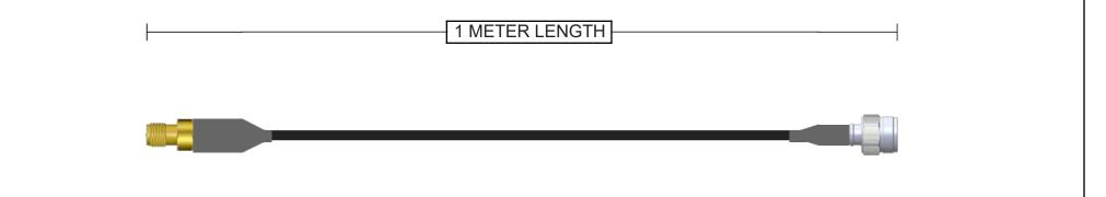
Connector A 132240RP SMA Jack Straight Brass Gold + Heatshrink 50 Ohm LMR-240 Continuity/Hi-Pot Connector B 031-6825 TNC Plug Straight Brass Nickel + Heatshrink
