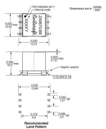
Packaging 350 per 13" reel Plastic tape: 24 mm wide, 0.5 mm thick, 16 mm pocket spacing, 10.4 mm pocket depth
