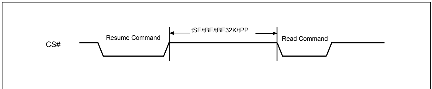
Figure 57. Resume to Read Latency
