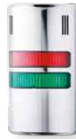
Order number: HD90-Q42 Colours: red/green Function: LED steady beacon, buzzer steady or pulsing tone Housing colour: chrome Nominal voltage: 24 V AC/DC
