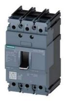
circuit breaker 3VA5 UL frame 125 breaking capacity class S 25kA @ 480 V 3-pole, line protection TM210, FTFM, In=15A overload protection Ir=15A fixed short-circuit protection Ii=20 x In UL489 SB (naval), 50 deg. cel. nut keeper kit on both sides
