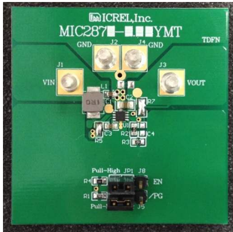
Figure 1. MIC2875-AYMT Evaluation Board
