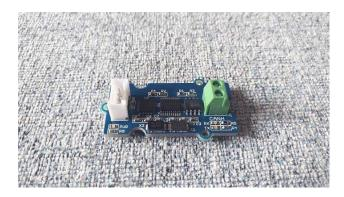
This Serial CAN-BUS module is based on MCP2551 and MCP2515, which can provide speed up to 1Mb/s.
