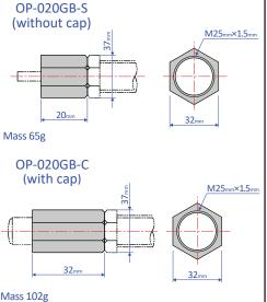
Note: When attaching, make sure that the side without a bearing chamfer is the impact surface.
