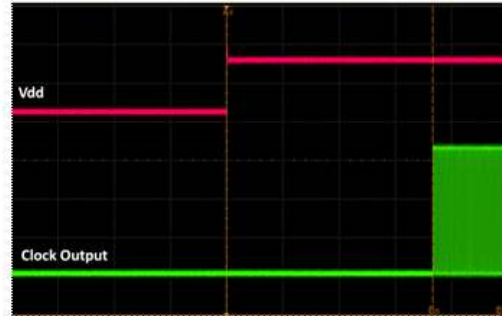
Figure 17. Startup Waveform vs. Vdd
