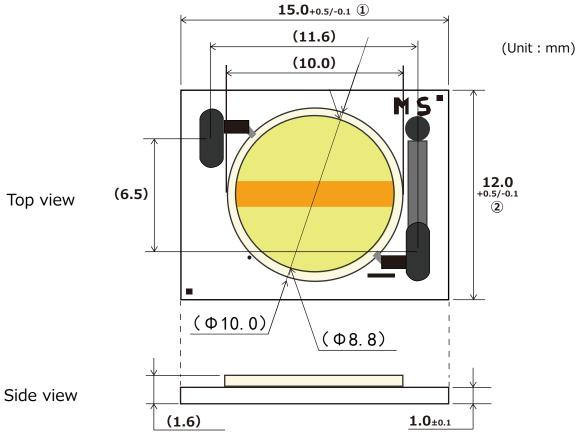
(Note) Values inside parentheses are reference values. External sizes of ①、 ② are determined by maximum dimensions, that include salient areas on the edges of respective sides.
