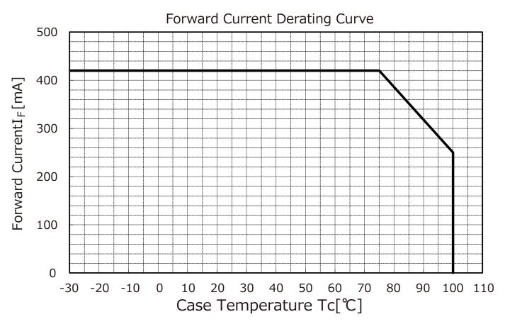
(Note) To keep the case temperature lower than the rating, enough heat-radiation performance needs to be secured by using an adequate heat sink.
