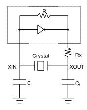
$C_L = 2^*(C_P - C_S), \\$  Where  $C_P = Load$  capacitance of crystal from crystal vendor datasheet.
