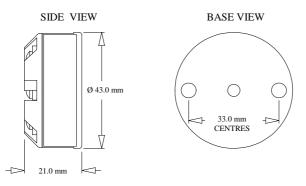
Fixing holes 2 x Ø5.5 mm, Centre hole Ø4.5 mm
