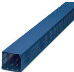
Wiring channel, blue, consisting of upper and lower part, width: 30 mm, height: 100 mm, length: 2000 mm
