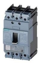
circuit breaker 3VA5 UL frame 125 breaking capacity class H 65kA @ 480 V 3-pole, line protection TM230, FTAM, In=90A overload protection Ir=90A fixed short-circuit protection Ii=5...10 x In cable connection on both sides
