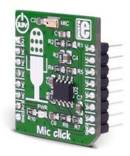
Mic click carries the SPQ0410HR5H-B surface mount silicon microphone with maximum RF protection. The click is designed to run on a 3.3V power supply. It communicates with the target microcontroller over the AN pin on the mikroBUS™ line.
