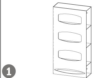
Mount securely to a wall with screws approved and supplied by building maintenance.
