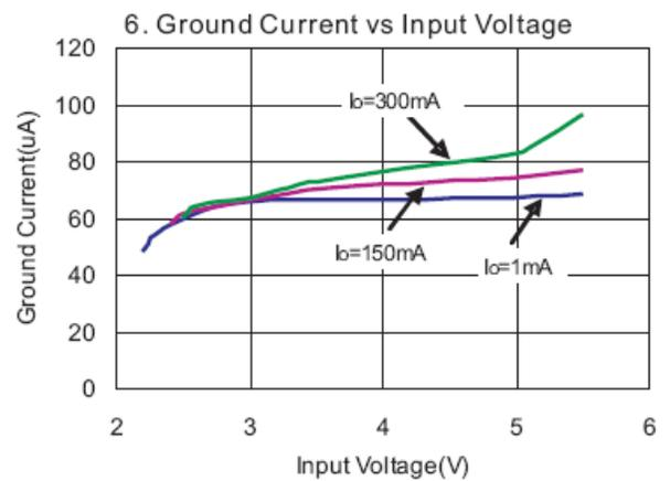
**Typical Performance Characteristics** (cont.) (@ $T_A = +25^\circ\text{C}$ ,  $C_{IN} = 1\mu\text{F}$ ,  $C_O = 2.2\mu\text{F}$ ,  $V_O = 1.2\text{V}$ , unless otherwise specified.)
