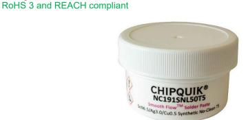
\*Shelf Life Notes: Chip Quik® solder paste is good past its quoted shelf life, regardless of refrigeration. Before use, visually inspect the solder paste to ensure it is not dried out or clumpy, or check stencil release. If stored in a jar, stir the product thoroughly for 2-3 minutes before inspection and use.
