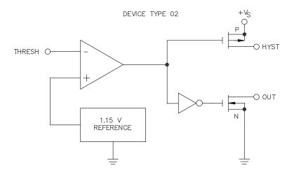
FIGURE 2. Block diagram.
