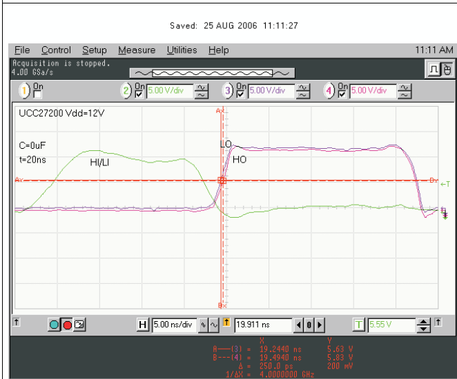
Figure 32. 20-ns Input Pulse Delay Matching
