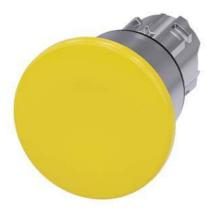
Mushroom pushbutton, 22 mm, round, metal, shiny, yellow, 40 mm, latching, pull-to-unlatch mechanism, with laser labeling, symbol number according to, ISO 7000 or IEC 60417
