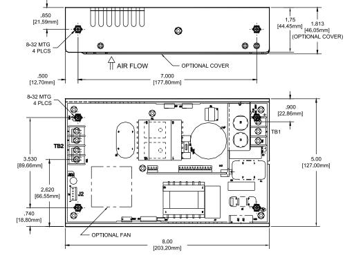
A. Units should be allowed to warm up/operate under non-condensing conditions before application of power. Derate output current and total output power by 2.5% per °C above 50°C.
