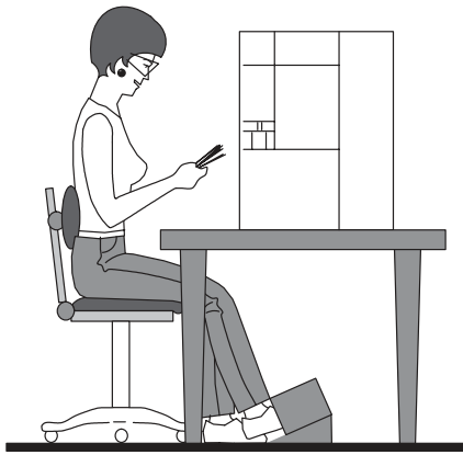
Figure 3 shows the physical considerations as recommended, and the operator in a desirable position. Note that the chair height and back rest are properly adjusted, and that the chair is properly located in respect to the bench. Thus, the operator's back is straight, and supported by the chair. Note also that the operator's upper arms are in a direct line with the torso.
