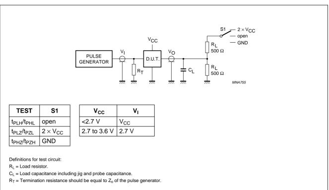
Fig.7 Load circuitry for switching times.
