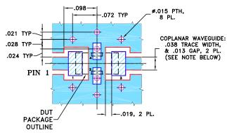
NOTES: 1. COPLANAR WAVEGUIDE PARAMETERS ARE SHOWN FOR ROGERS RO4350B WITH THICKNESS .020" ± .0015". COPPER: 1/2 OZ. EACH SIDE. FOR OTHER MATERIALS TRACE WIDTH & GAP MAY NEED TO BE MODIFIED.
