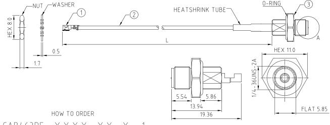
(AB463RF - X X X X - X X - X - 1 SMA DETAIL DRAWING CABLE SIZE OPTION: "L" LENGTH IN MM:  $1 = \phi 1.37MM$  CABLE, COLOR: BLACK eq: 100MM = 0100(MIN. 0050-MAX.0400 STANDARD = 0100, 0150, 0200) WASHER AND NUT OPTIONS: Tolerance: 50-200mm: ±5mm.
