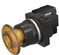
30mm BlackMax, Epoxy Coated Corrosion Resistant Complete Metal Unit Illuminated Push-Pull Operator Full Voltage, 12V AC/DC Incandescent Lamp Mushroom Head Cap Small 1 3/4" (44.5 mm) Plastic, Amber 3 Position Pull-Momentary/Push-Maintained UL Listed, CSA Certified NEMA 1,3,3R,4,4X,12,13 & Automotive Standards
