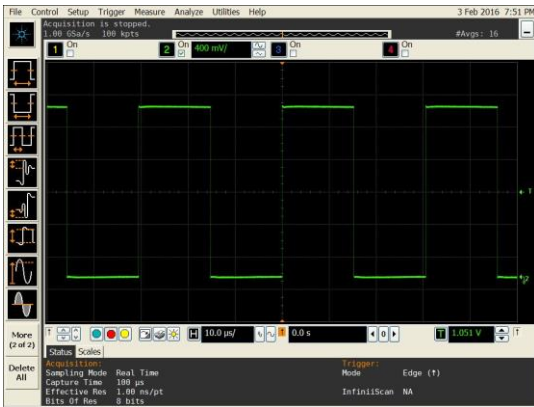
Figure 3. LVC MOS Output Swing ( V_{DD} = 1.8\text{ V} )
