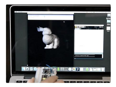
Also notice in the upper right corner of the dialog box at the top that the calibration of each sensor is displayed. It's important to calibrate the BNO055 sensor so that the most accurate readings are retrieved. Each sensor on the board has a separate calibration status from 0 (uncalibrated) up to 3 (fully calibrated). Check out the video and information from this guide for how to best calibrate the BNO055 sensor ().
