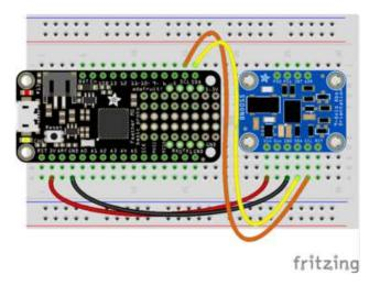
Board 3V to sensor VIN Board GND to sensor GND Board SCL to sensor SCL Board SDA to sensor SDA
