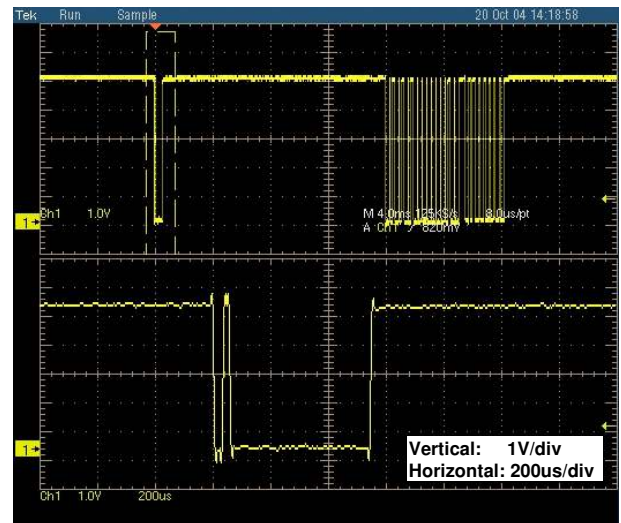
FIGURE 14. POWER-ON BREAK SIGNAL TO WAKE-UP THE ISL9206 FROM SLEEP MODE
