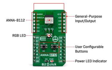
By integrating most of the critical components on the chip, the ANNA-B112 allows the module to overcome any imperfections of external discrete components, allowing signal transmission power of up to 5dBm, and -92 dBm sensitivity for the receiver, using the on-chip antenna.
