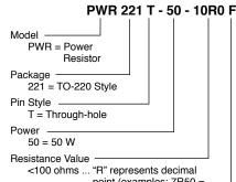
point (examples: 7R50 = 7.5  $\Omega$ ; R500 = 0.5  $\Omega$ ) ≥100 ohms.... First three digits are
