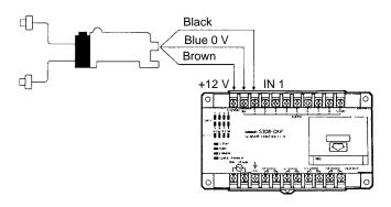
Note: A maximum of two E3X Optical Fiber Photoelectric Sensors can be connected.
