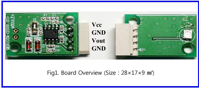
Fig1. Board Overview (Size : 28x17x9 mm<sup>3</sup>)
