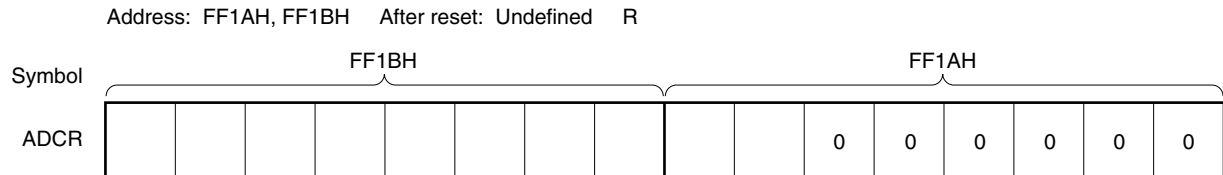
Figure 13-6. Format of A/D Conversion Result Register (ADCR)
