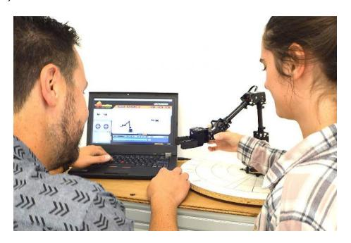
Given that the structure of the arm is comprised of modular brackets and servos, purpose-built and ultralight aesthetic plastic shells give a futuristic look to the arm without impeding any motion. The shells are held in place using neodymium magnets, and vinyl stickers allow for personnalisation.
