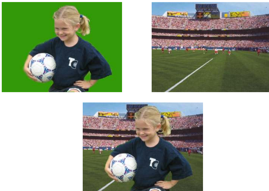
Figure 17-13. Pixel Pipeline (PXP) Colorkey Example
